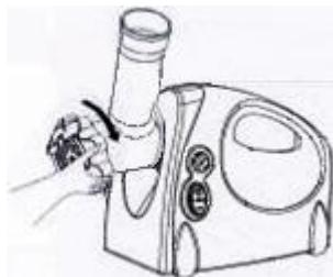
6. Place the hopper plate on the grinder head and fix it.
