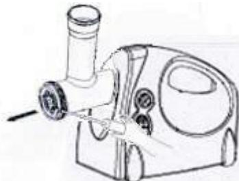
In order to take the grinder head off the meat grinder - press the lock button and turn the grinder head clockwise. Remove the feed screw from the grinder head by pulling it or after removing the grinder head from the meat grinder, push the feed screw from the back side.
