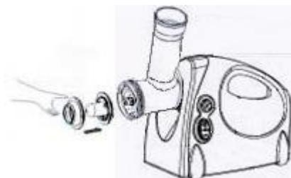
3. Tighten the cap, but do not tighten it excessively. Set the hopper plate on the grinder head and fix it.
